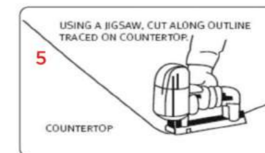
5 Using a jigsaw, cut along the inside line to cut the opening in the countertop.
