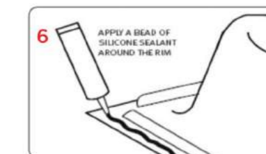
6 With sink in the upside down position, place a continuous and generous bead of silicone sealant around the entire perimeter of the rim. This serves as a watertight seal.
